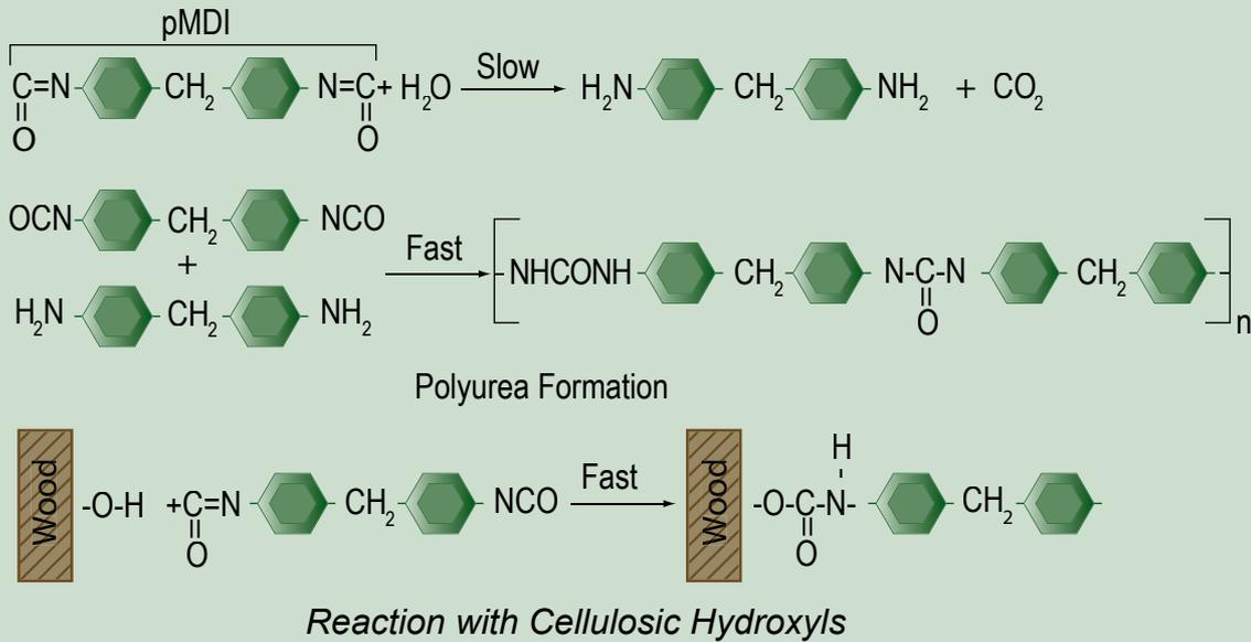
pMDI is not thermoplastic, it will not reverse the thermoset achieved during the curing process in the press, unlike some other bonding resins that are thermoplastic and are reversible due to heat, thus losing their bond. The resin is also unaffected by UV light and water.
